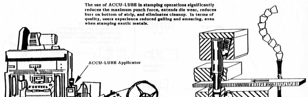
Stamping applications using ACCU-LUBB require a two-nozzle applicator. Position the nozzles above and below the workpiece prior to the strip entering the die sets. Surface coating the strip with ACCU-LUBB allows lubricant to be drawn into the punch and die/workpiece interface.
