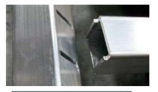
Slot and tab construction greatly reduces measuring, welding & assembling times
